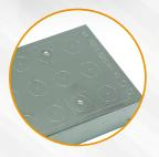
KING Tester Test Blocks are traceable, serialized, affordable and meet ASTM E-10 standards of 1% tolerance. Our patented, etched, crosshair design improves test accuracy.
